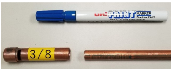
FIGURE 24: Pipe Marking Tool and Paint Marker
