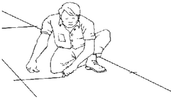
FIGURE 5: Measure and Mark Exact Case Outline
