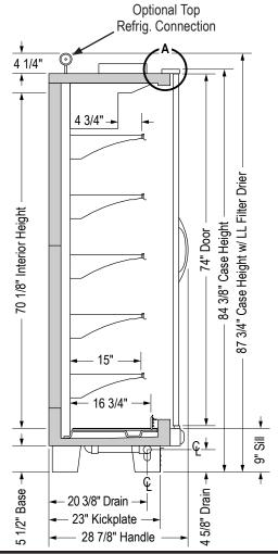
**IMPORTANT: The Ultra Narrow must** be anchored to either another case or a wall to ensure the case will not tip forward. See Installation & Operation Manual for more information.
