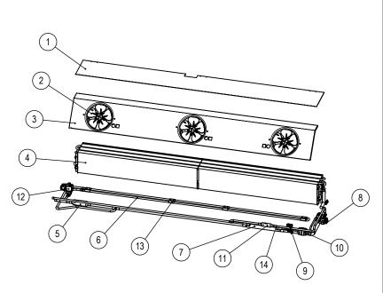
FIGURE 50: Hot Gas Defrost Components
