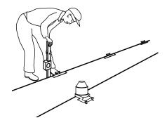
5. If your case uses optional hat channel rails to raise the case height, place shims *under* the hat channel rails (See Figure 6 on page 7). On 3 and 4-door cases, the center bases are not aligned, so the hat channel rails must be angled slightly to support the bases; do not position hat channel rails under the drain hub (See Figure 7 through Figure 9 starting on page 7).
