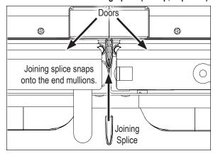
FIGURE 15: Vertical Joining Splice (V-Strip, Front View)
