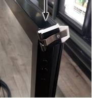
FIGURE 29: Remove Torque Rod
