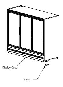
Shims must be placed under the front and rear bends of each base to prevent the base from warping/buckling.
