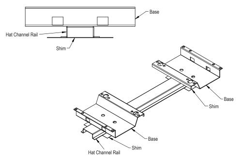
Position hat channel rails with tape up. Place shims perpendicularly under the hat channel rails.
