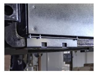
**FIGURE 3: Spacer Block**
