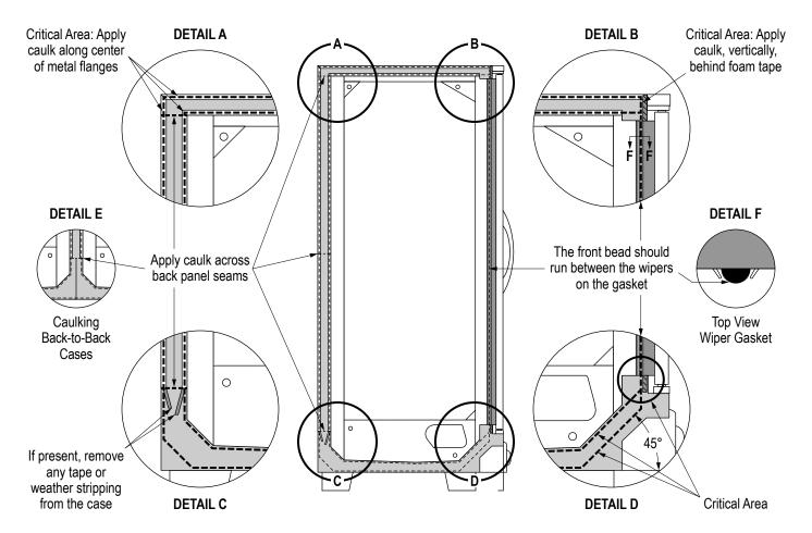
FIGURE 16: Case Joint Caulking (Butyl\*)
