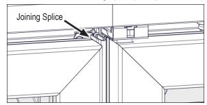
Before joining the cases, remove all packaging material on the display case, including any spacer blocks inside the bases. Repeat caulking between each case in the lineup.
