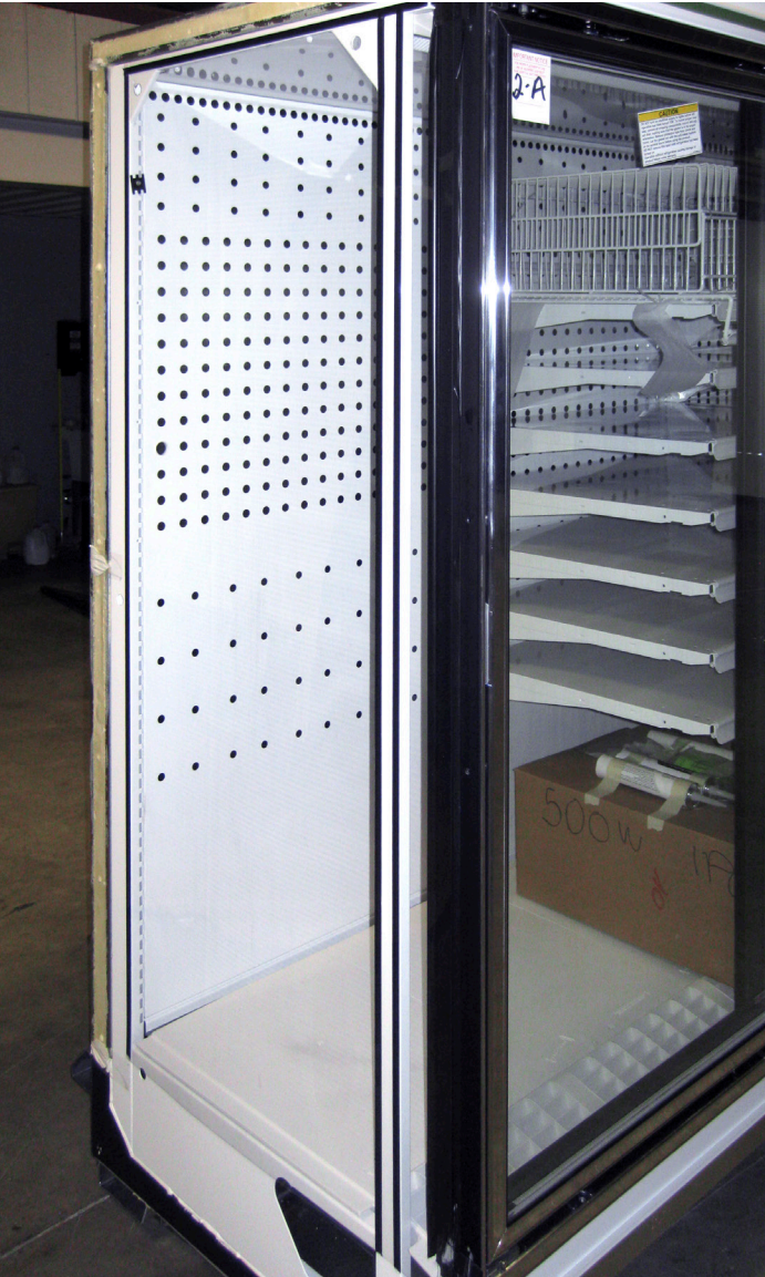
Clear plexi dividers separate refrigeration circuits between same-temp cases.
