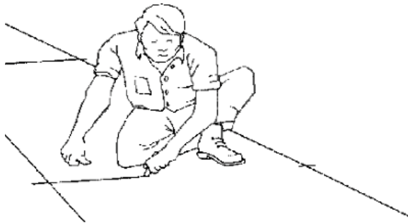
FIGURE 5: Measure and Mark Exact Case Outline
